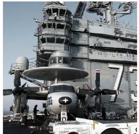
▲ ISLAND SUPERSTRUCTURE Much of the electronics, including radar and satellite-communications equipment, is based on the island, which has the ship's number painted on its sides.
